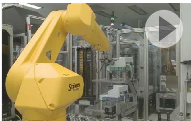
Next, the robot arm moves the plate from the incubator to a pin-tool device, where chemicals dissolved in a solvent are transferred into each well. There is a different 1,536-well plate for each concentration. The total number of plates in each run depends on the number of chemicals and the number of concentrations being tested.
