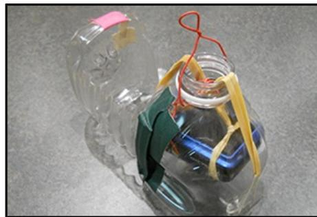
Wylie's homemade satellite includes a reused plastic juice bottle, rubber band harness, and inexpensive digital camera, which can detect hydrogen sulfide contamination and map thermal pollution. (Photo courtesy of Joe Balintfy)
