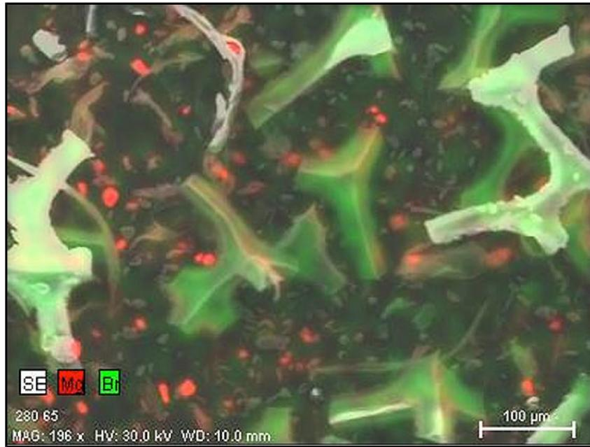
*Researchers used a scanning electron microscope with energy-dispersive X-ray spectroscopy to create an image of the dust from a gymnastics foam pit. The presence of brominated flame retardants in fragments of foam are indicated in green. Red indicates magnesium, presumably from gym chalk. (Photo courtesy of Simon C. Roberts, Duke University)*
