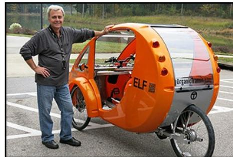
*Fannin is proud of his eye-catching new machine. The mirrors, lights, and turn signals on the ELF, along with physical protection from all but the worst natural elements, make it much safer than a bicycle. (Photo courtesy of Richard Sloane)*
