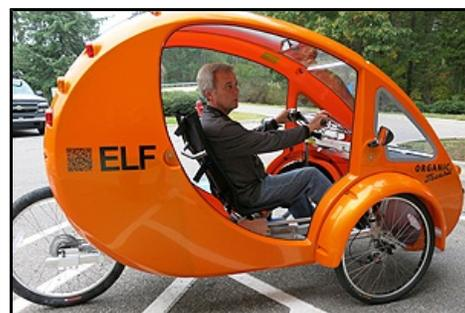
*According to Fannin, the ride is very much like a bicycle. The big difference is the assistance of a small electric motor for getting up hills and maintaining a good speed - approximately 20 mph - with the velomobile, which weighs about 115 lbs. The vehicle is fun to drive and comfortable in the recumbent seat, but, without shocks or springs, it doesn't always offer a smooth ride. (Photo courtesy of Richard Sloane)*
